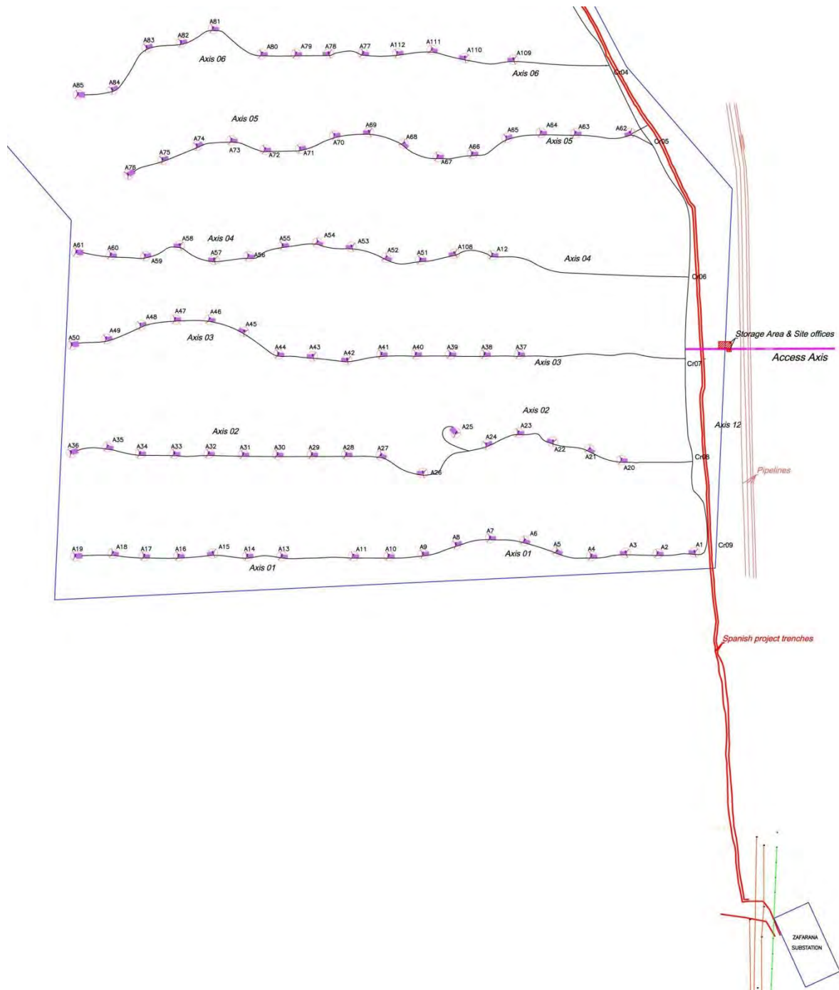
Fig. 2.5: Typical Arrangement of Wind Park Siting Kiosks and cabling to 220 kV SS
