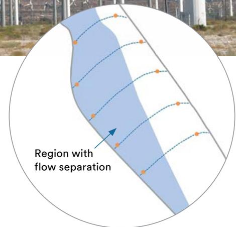
Example of a flow separation region for a specific blade type. Its border corresponds with the 3M Wind Vortex Generator installation line.
