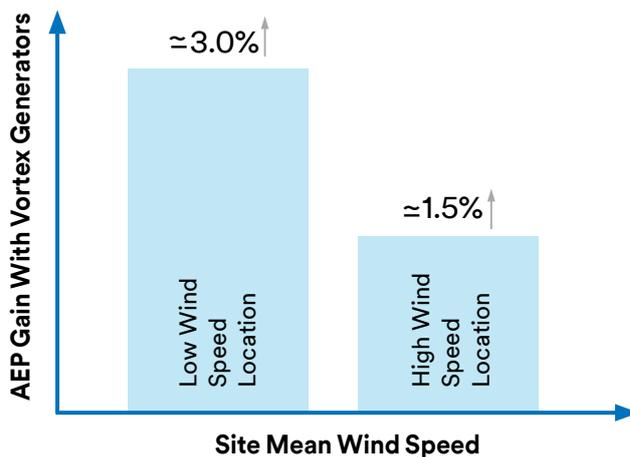
Optimizing blade aerodynamics helps achieve a significantly higher energy yield, for higher profitability. The increase is dependent upon the turbine site, the turbine type and the turbine condition. Long-term field tests show increases in annual energy production of 2.0% or more.
