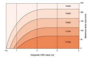
With a soft subgrade it is prudent to place at least 300mm of lightlycompacted sub-base in one lift (500mm on an exceptionally soft subgrade) before overlaying this with a thinner layer of bettercompacted material.
