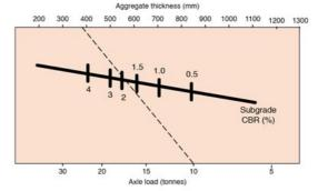
Example: Subgrade CBR = 2%, Axle load = 10 tonnes, Stone thickness required = 350m
