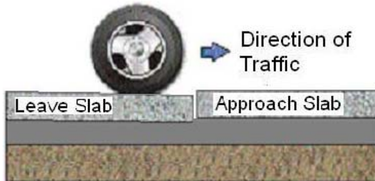
Figure 7. Slab Movements in Non-doweled Slab
